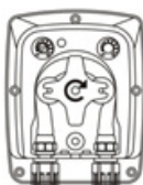
While turning rotor install tube in race
