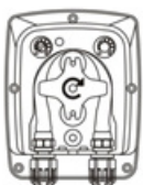
Align rollers at "12 and 6"
